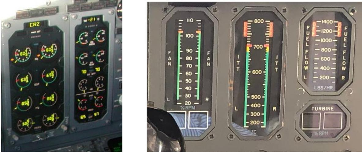
Figure 3. "Round-dial" and tape electronic engine displays.
