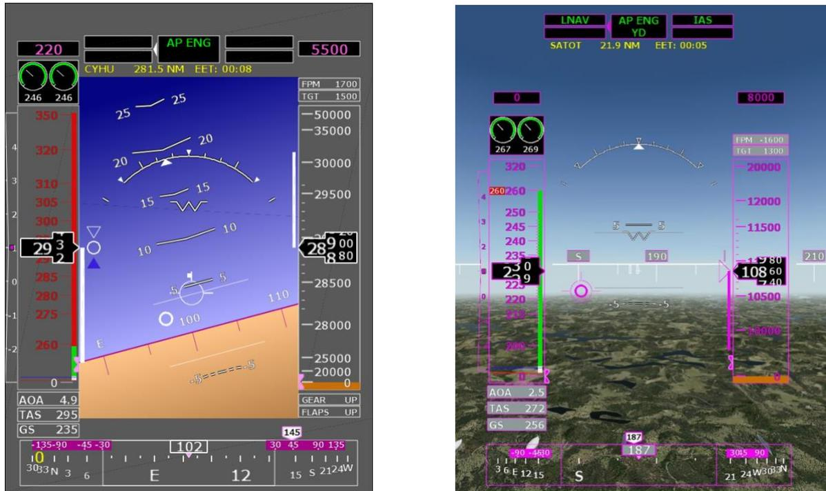
Figure 5. DNLD PFD and SVS displays.
