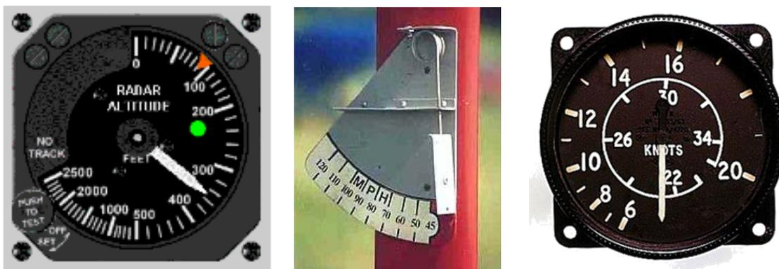
Figure 2. "Classic" non-linear radar altitude and airspeed displays.
